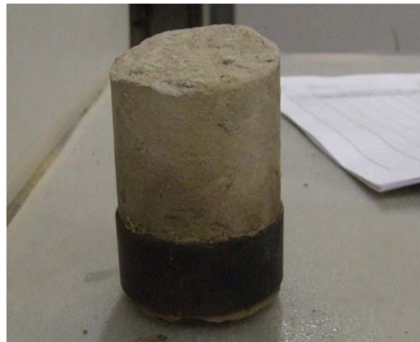
Figure 2. HQ core and test ring
