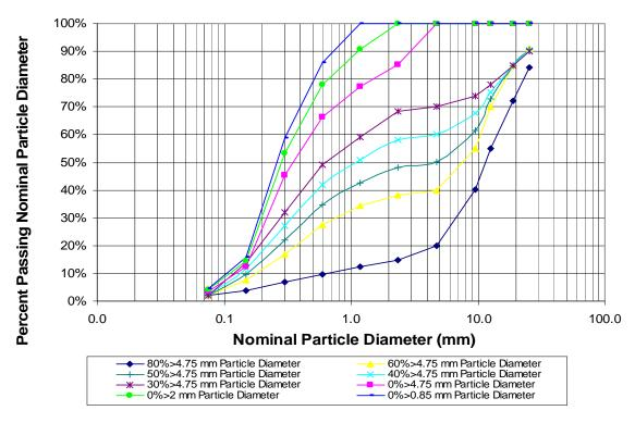
Figure 3. Particle size distribution of fabricated soils.
